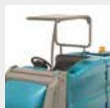
**FOPS certified overhead guard** protects operators from falling objects.
